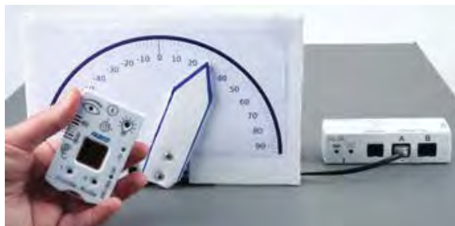
A stepper motor rotates the meter indicator to match the angle at which the //code.Node is tilted.
