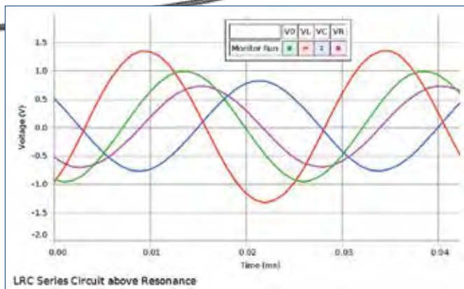
The oscilloscope display in PASCO Capstone is used to simultaneously display the voltages across the inductor, capacitor, and resistor, as well as the source voltage.
