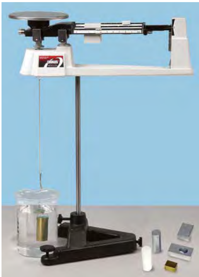
The mass and volume are measured to determine the dependence of the buoyant force on mass, volume, and density.
