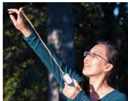
The Wireless 3-Axis Acceleration/Altimeter is launched by a stretched rubber band that is connected to one of the many attachment holes in the rubberized case. The graph shows the resultant acceleration (measured in g's) and the altitude for the four-second flight.
