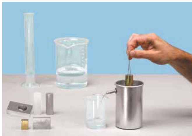
The buoyant force is measured by weighing the water displaced by the object.
