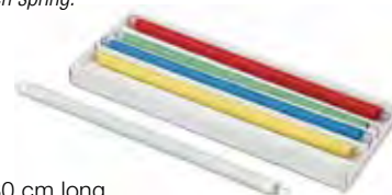
The five color-coded springs stretch different amounts when a 1 kg mass is hung from each spring.
