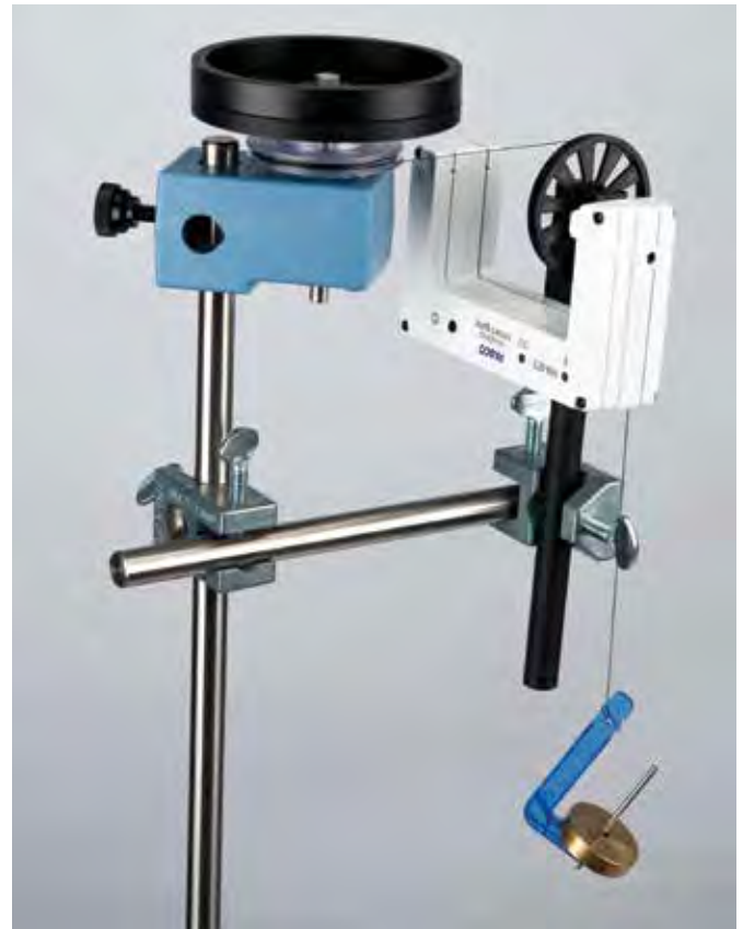
A Smart Gate with a Pulley measures the rotational velocity of the apparatus mounted on the Pivot.
