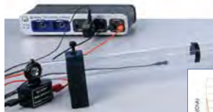
The included auxiliary microphone can be used to probe a resonance tube.
