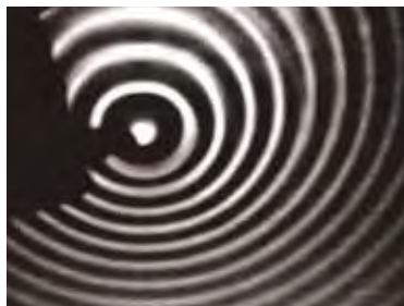
The Doppler effect is clearly demonstrated by moving the dipper. In this picture the movement is downward.
