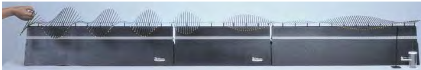
The complete Wave Motion Demonstrator in three sections: The high-amplitude, slow-moving waves provide a fascinating introduction to basic wave phenomena.
