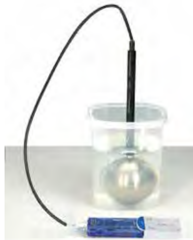
Measure the pressure and temperature of air in the sphere.
