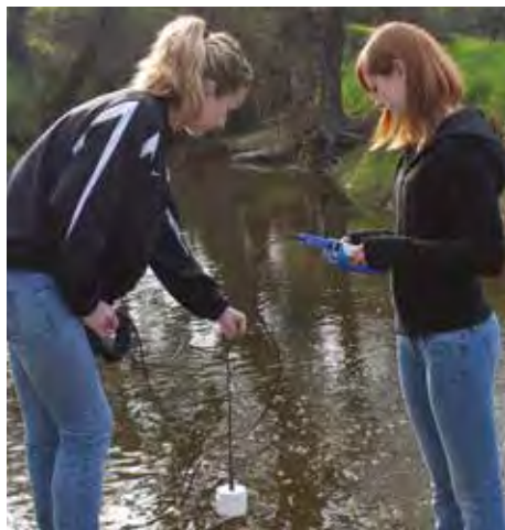
The temperature of the water in a pond is measured as a function of depth.
