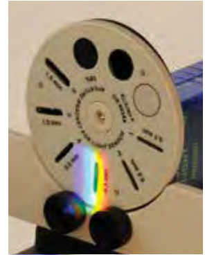
The continuous blackbody spectrum is scanned using a prism spectrophotometer.
