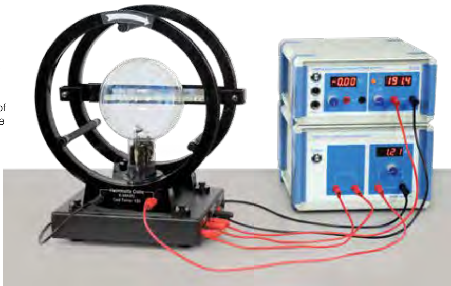
The complete Charge-to-Mass Ratio System includes the power supplies, which can also be used in other experiments (such as the Franck-Hertz experiment, see page 389).
