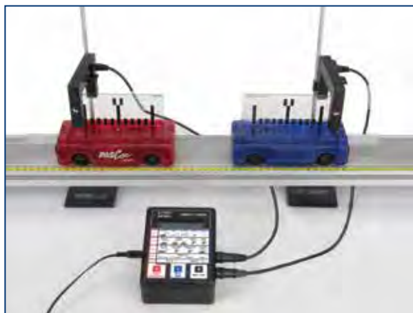
Speed before and after collision—In Speed: Collision mode; use two carts and two photogates with a single Smart Timer to measure initial and final speeds of both carts.
