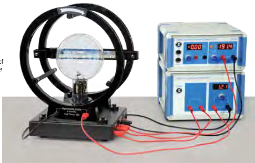
The complete Charge-to-Mass Ratio System includes the power supplies, which can also be used in other experiments (such as the Franck-Hertz experiment, see page 404).
