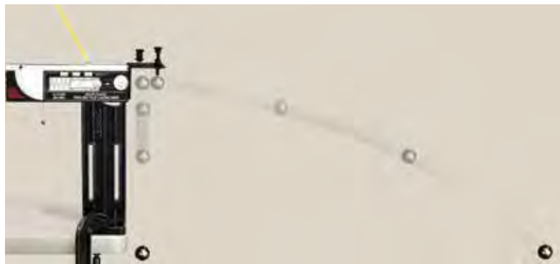
When the solid ball hits the hanging solid ball, the hanging ball shoots out horizontally, while the ball shot out of the launcher drops straight down.
