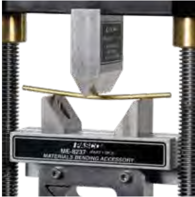
A Three-Point Bend Test is performed on a brass rod from the ME-8240 Shear Samples. The support anvils have adjustable separation up to 10 cm.
