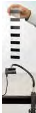
Flex Rod holds photogate for Acceleration Due to Gravity experiment using a picket fence (shown with Table Clamp, not included).
