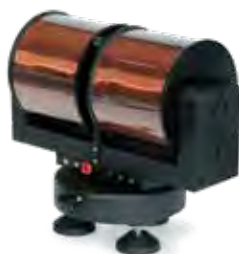
Electromagnet produces about one Tesla.
