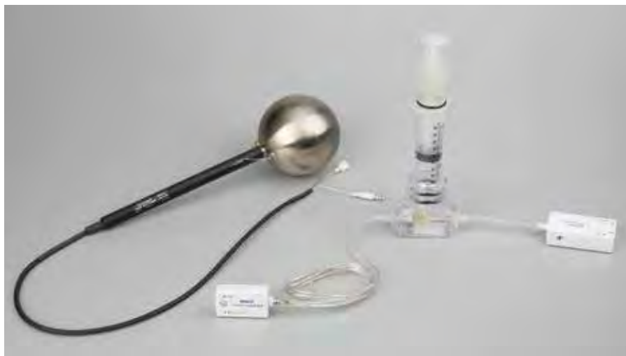
For the Ideal Gas Syringe (shown above) the slope of the Pressure vs. Inverse Volume is nRT .
