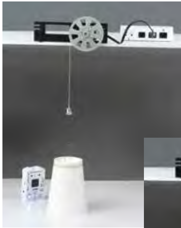
Light reflected from the cup triggers the winch to lower.
