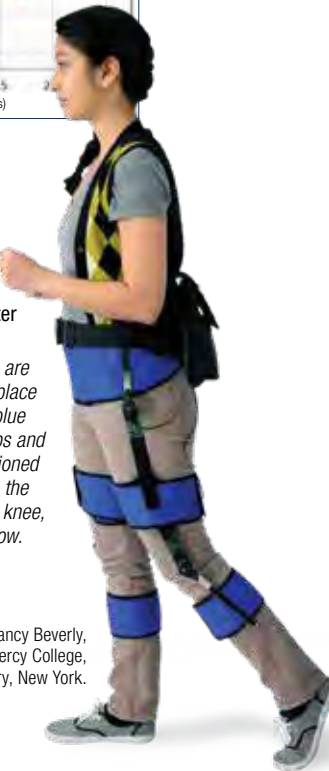
Data shows position of both left and right knee and hip joints during walking.
