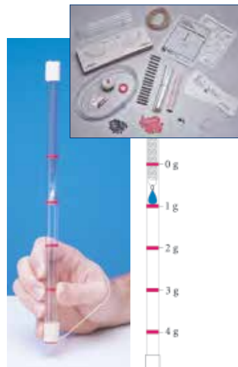
Vertical Accelerometer: The stretch of the spring measures the vertical acceleration in "g's."
