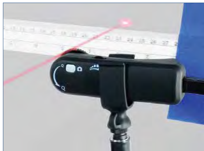
The USB Camera Microscope records the oscillation of the laser beam reflected off the Gravitational Torsion Balance (AP-8215A).
