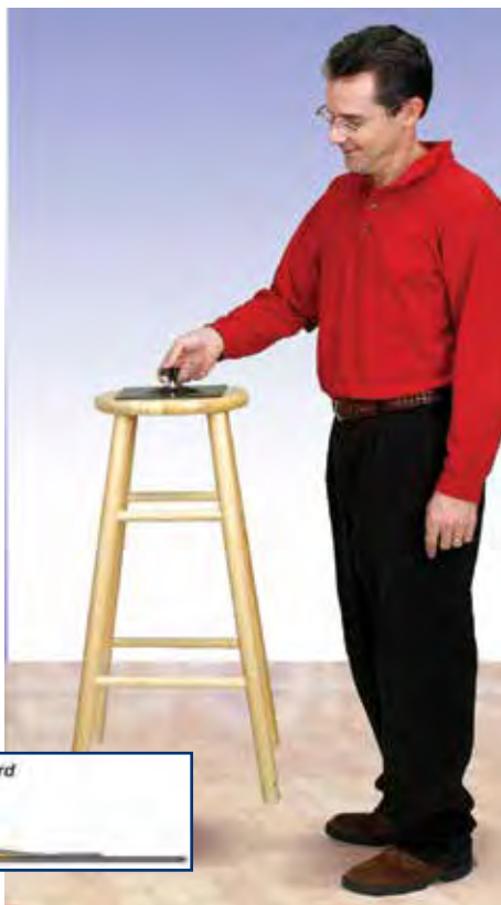
As you pull up on the handle, a low-pressure region is created.
