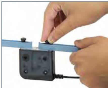
I-Beams key into the Load Cell and are fastened with thumbscrews.
