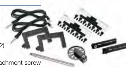
Position and velocity graphs are obtained using a Picket Fence and Photogate.
