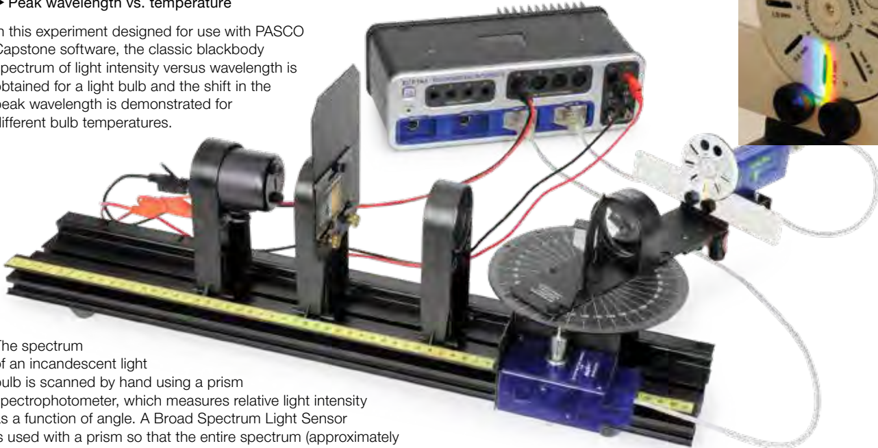
The continuous blackbody spectrum is scanned using a prism spectrophotometer.
