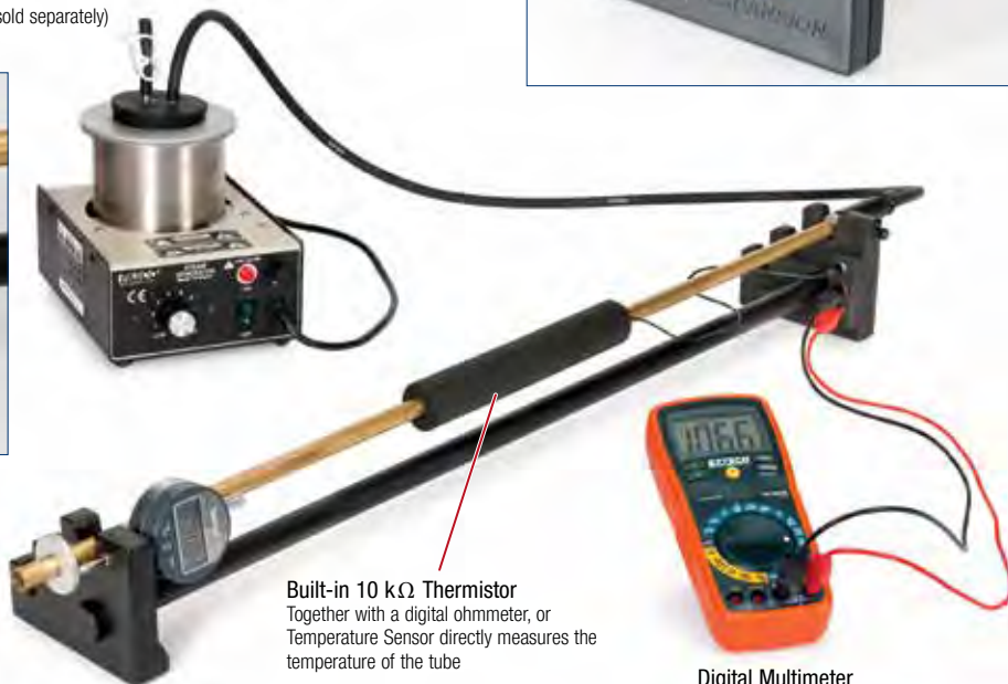
Digital Multimeter Measures thermistor resistance (sold separately)
