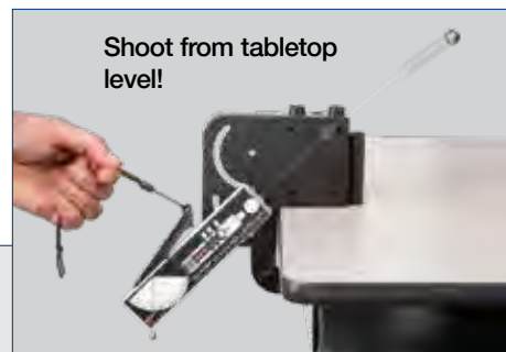
Unique stand design allows ball to be launched from tabletop height. The ball lands on the table at the same height from which it was launched.
