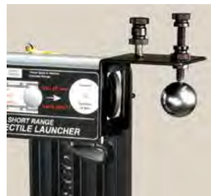
Either the solid steel ball or hollow steel ball is hung by a magnet.
