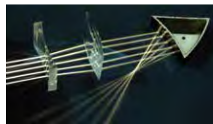
Components from the Ray Optics Kit showing refraction and reflection
