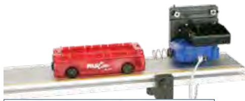
Use it with the Wireless Force Acceleration Sensor (PS-3202) to study cart collisions.
