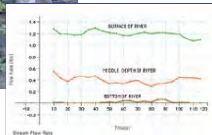
Graph shows the flow rates at the top (green), middle (orange), and bottom (brown) of a stream.
