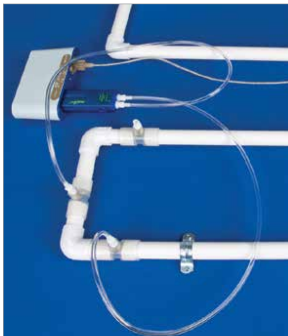
Study one pump or two pumps in series and parallel.
