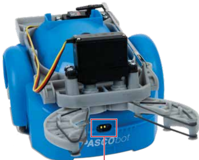
The Range Finder Lidar infrared emitter/detector pair peeks through a hole in the front of the PASCObot.
