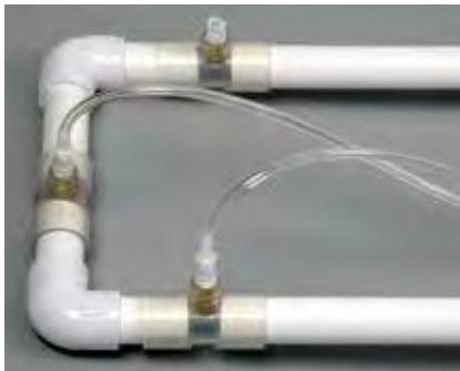
Instrument your pipe network with the Pressure Taps connected to the Dual Pressure Sensor (PS-2181).
