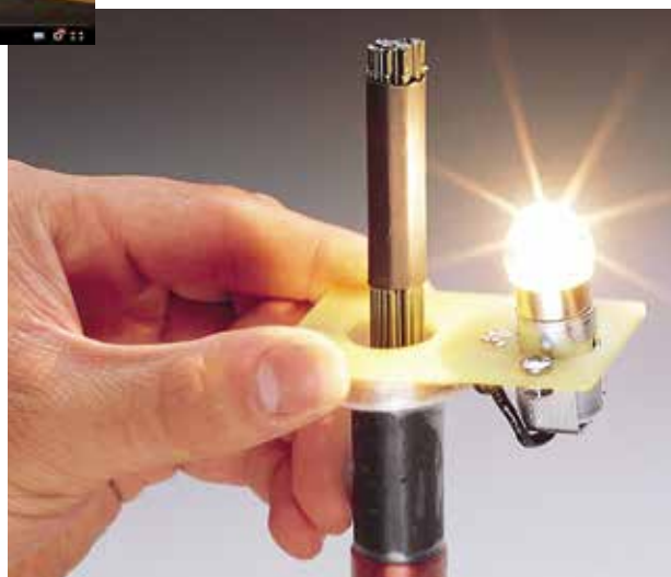
Lighting a bulb connected to a coil by induction; coil and bulb are included in Ring Launcher Accessories.
