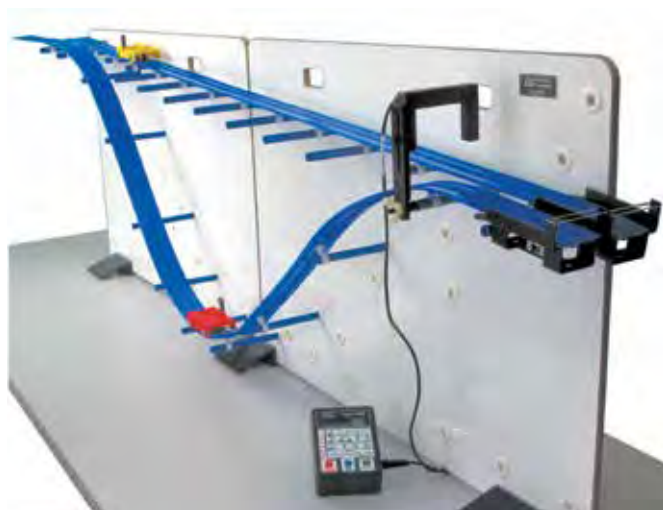
Conservation of energy shows that the final speeds of these two cars are the same even though the red car takes much less time than the yellow car to reach the end of the track.
