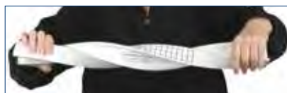
Demonstrate lack of torsional strength.
