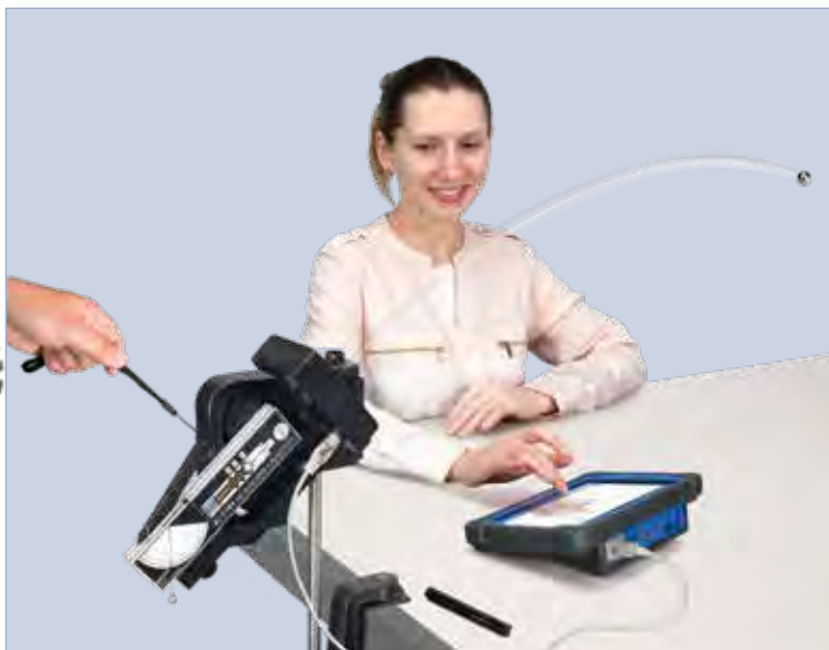
The launch speed of a ball launched by the Mini Launcher is recorded by a Smart Gate attached to the SPARK LXi2.
