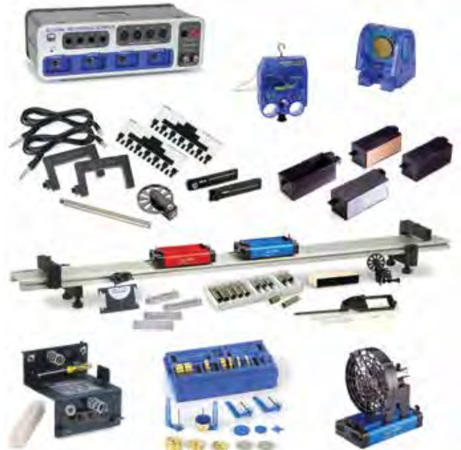
Impulse Experiment Measure the force as a function of time as the cart hits the spring and also measure the change in momentum using the photogate.
