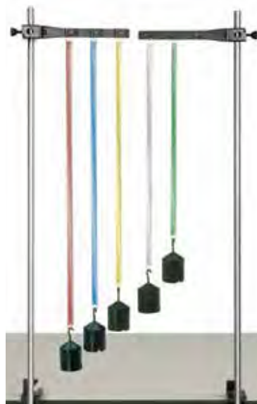
The five color-coded springs stretch different amounts when a 1 kg mass is hung from each spring.
