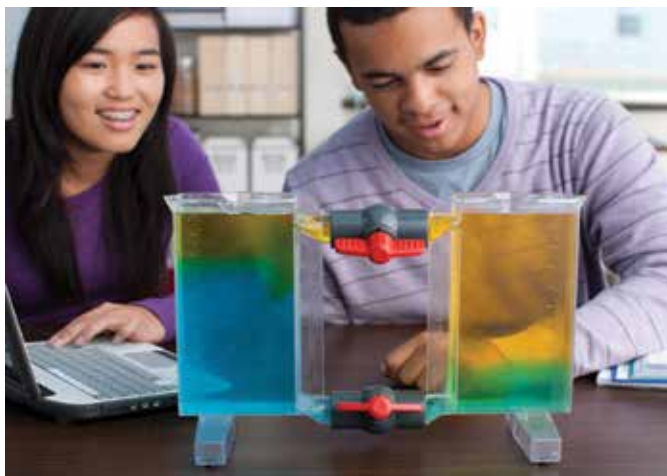
As students open the valves, convection-driven circulation begins and the water types begin to layer—even for very small temperature/density differences.
