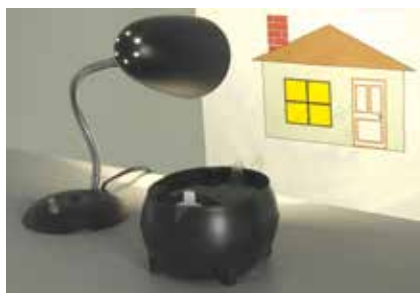
The Human Eye Model can image any illuminated picture.
