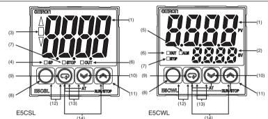
(1) Display No. 1 Displays the process value (PV) or parameter. For the E5CSL, the set point or parameter setting is also displayed. Displays the set point (SP) or parameter setting. (2) Display No. 2
